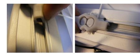
Press one leg in the profile. Press the other leg in the profile after that.
