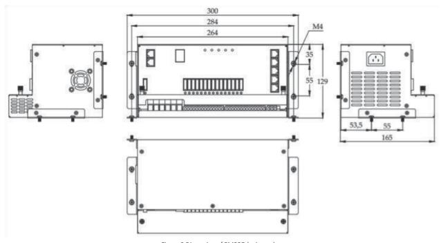
Figure 9 Dimension of PM235 (unit: mm)
