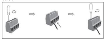
Figure 19 Connection of Terminal Type 1
