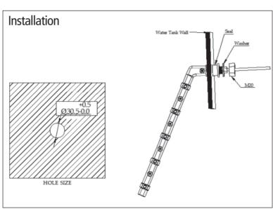
Figure 14 Installation of PMWS400
