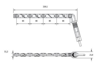
Figure 15 Dimension of PMWS200 (Unit: mm)
