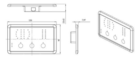
Figure 11 Dimension of PMSWLED (Unit: mm)
