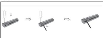
Figure 20 Connection of Terminal Type 2
