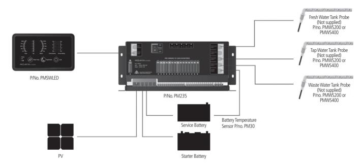
Figure 1 System Components for PM200
