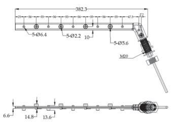
Figure 13 Dimension of PMWS400 (Unit: mm)
