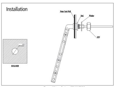
Figure 16 Installation of PMWS200
