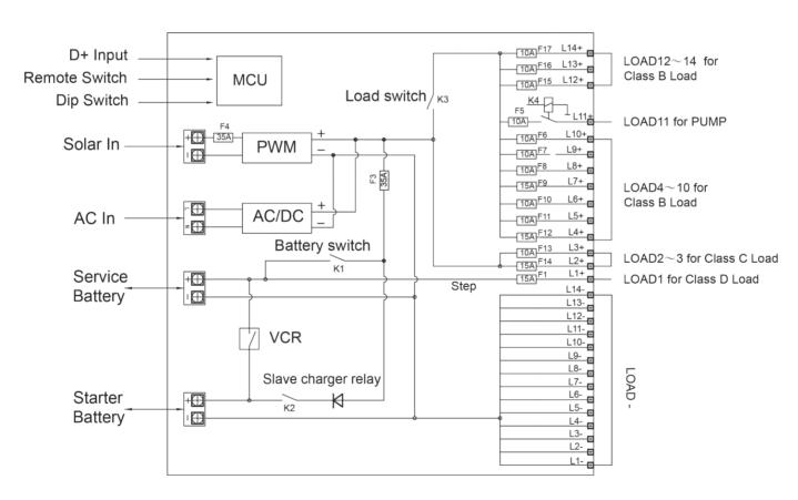
Figure 2 System Schematic
