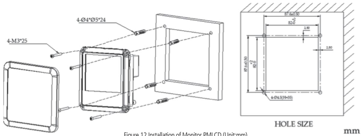
Figure 12 Installation of Monitor PMLCD (Unit:mm)
