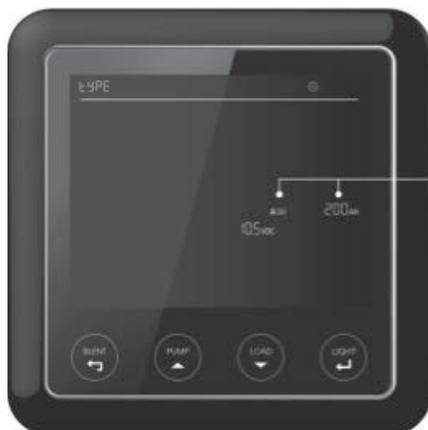
When the battery type and capacity setting on the monitor is not the same as PM335 dip switch, the icons will be flashing.
