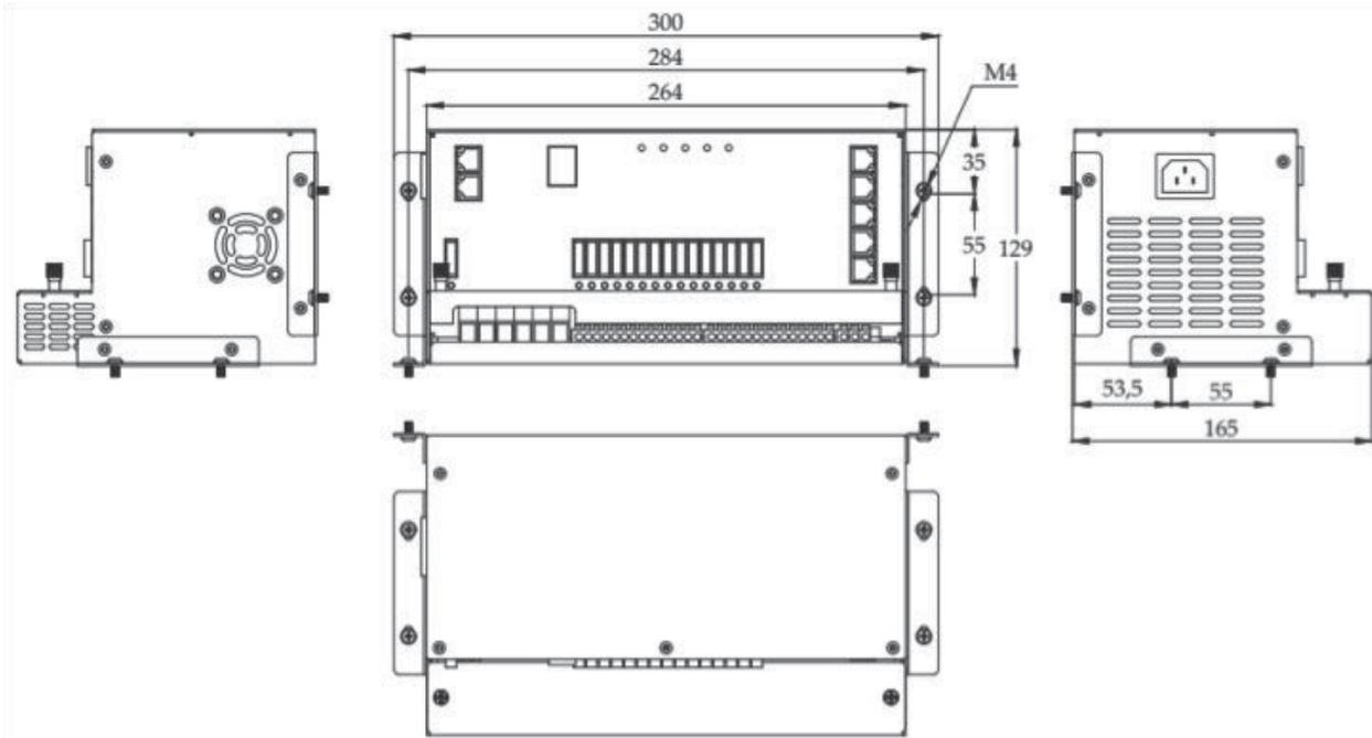
Figure 9 Dimension of PM335 (Unit: mm)
